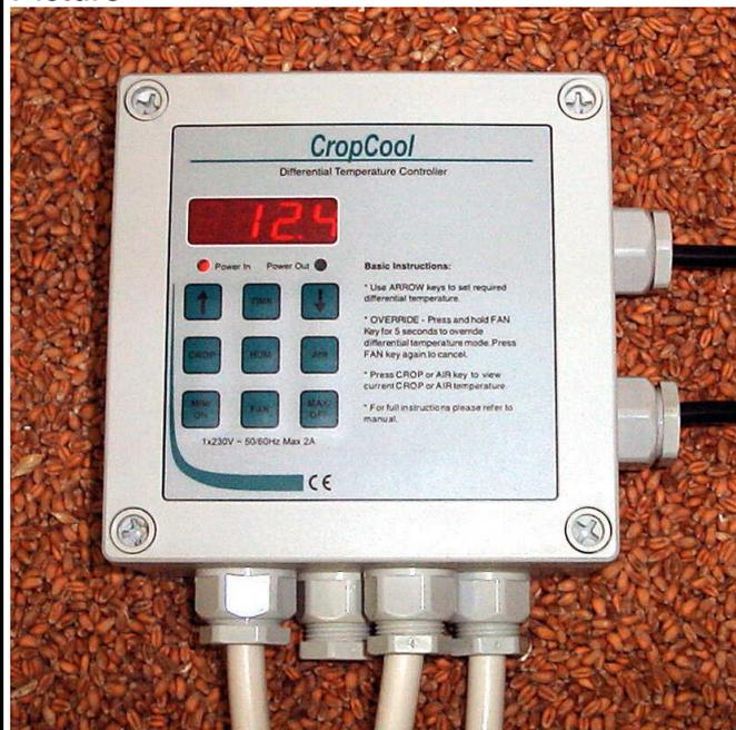
In addition to the display there are 2 **LED's** which indicate when there is power going to the controller and when the sockets are switched on.
